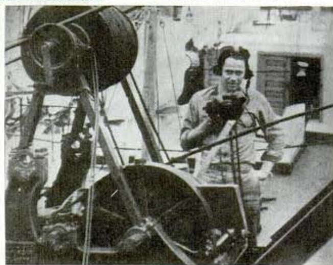
Below, talking by phone from deck of salvage vessel to diver on sea floor
